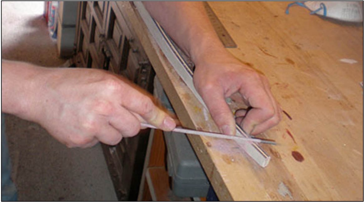
Picture 43: A chain saw file has exact the right size for the string grooves
