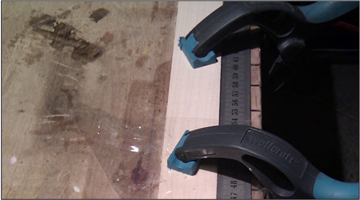
Picture 33: With a pair of clamps we fix the lams in place while the glue is curing
